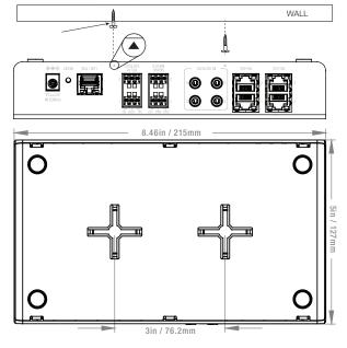
**NOTE:** Mounting height < 2 meters. Weight < 1 kg.
